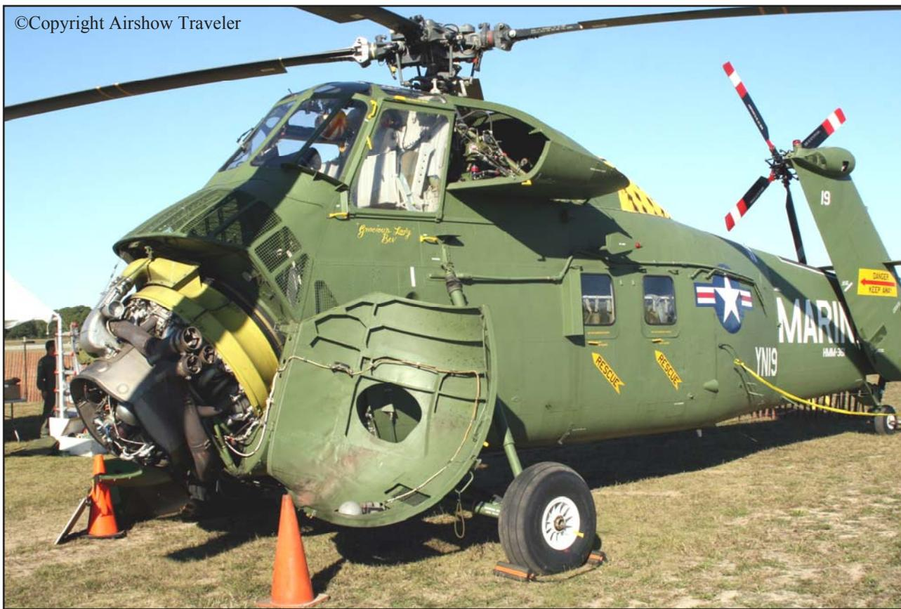
YN19 on display at the Grand Old Air Show, with its engine compartment doors open showing off its Wright R-1280-84 radial engine and massive cooling system.
